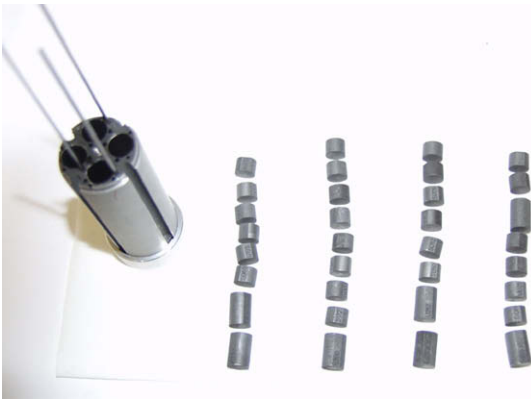
Fig. 3. A metal drum with four stacks to load the graphite specimens.
